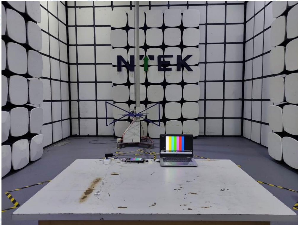
Radiated Measurement Photo
